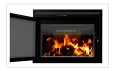
Our products have a unique design that allows secondary air to enter through a perforated baffle offering an unimpeded viewing area to the fire all while increasing the stove's efficiency and prolonging the combustion.
